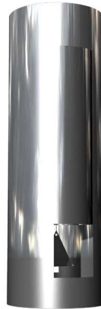
Exterior View 3"-diameter bell housed inside a 4"-diameter cap with vertical slot for wind flow
