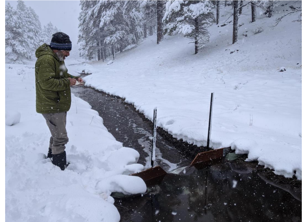
Aquifer seepage study 3/19/2020. Allen Haden, Natural Channel Design, documents the 1,000 gallons-per-minute release of reclaimed water at Lonetree at Bow & Arrows Wash.
