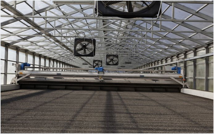
SOLAR DRYING IS A “GREEN” ALTERNATIVE THAT CAN ACHIEVE CLASS A BIOSOLIDS AND IS AMENABLE TO FLAGSTAFF’S ENVIRONMENT
