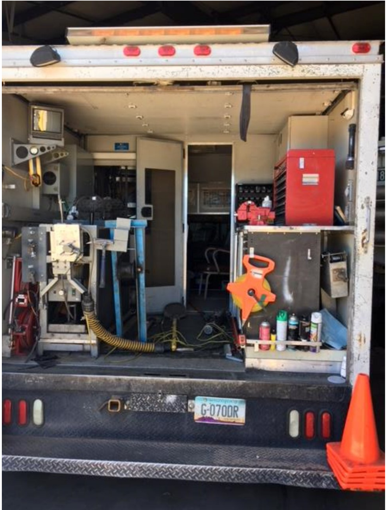
Equipment Area of existing Video Inspection Van S4030
