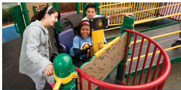
Balcony decks are recommended to increase the amount of toe space for a frontal approach to the reach panel — thus enhancing access and safety.
