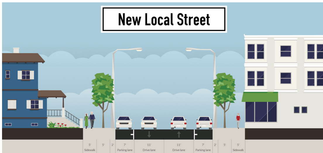
Figure 20: Cross-Section of New Local Street (60 foot right-of-way)
