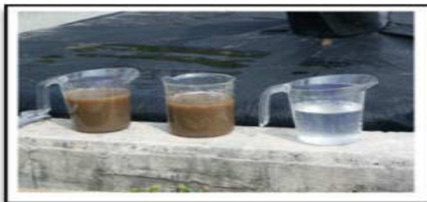
Raw digester sludge (left), treated with polymer (middle), and effluent from Geotube (right)
