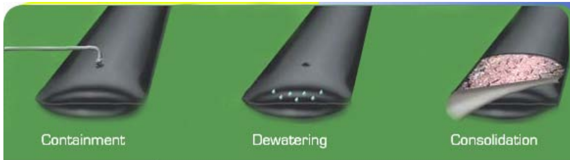
Figure 5 Three Stages of Geotube Dewatering Process
